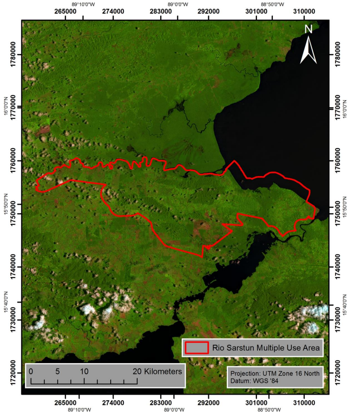
Figure 5: Landsat 8 scene (28/02/2014; bands: short wavelength infrared (band 7), near infrared (band 5), and red (band 4) used for the mangrove and seagrass mapping.
